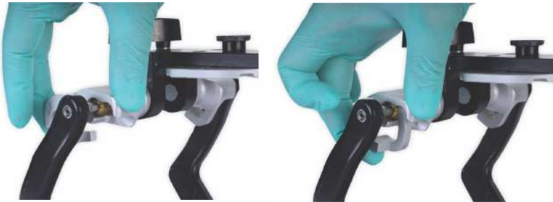
Fig. 8.24, 8.25: Centric latch holding the condylar ball in centric relation. In this position, the articulator can only make hinge movements along the terminal arc of rotation. Note: This does not mean that the articulator or mandible is restricted to this centric relation axis of rotation. Both, the mandible and the articulator are free to hinge around any axis and move into any translatory position. However, locking the condylar ball precisely 'co-relates' a 'recordable' and 'repeatable' hinge axis position on the articulator, allowing us to alter the vertical.
