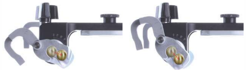
Fig. 8.52, 8.53: A flatter horizontal condylar guidance angle (left) and steeper angle (right). Note the altered path taken by the condylar ball during translation.
