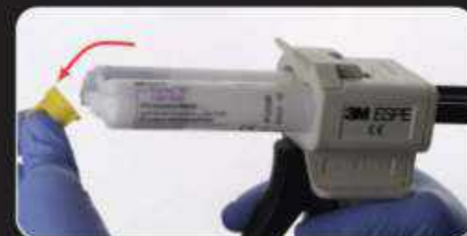
Fig. 5.64: The cap is then released from the cartridge using firm downward pressure.
