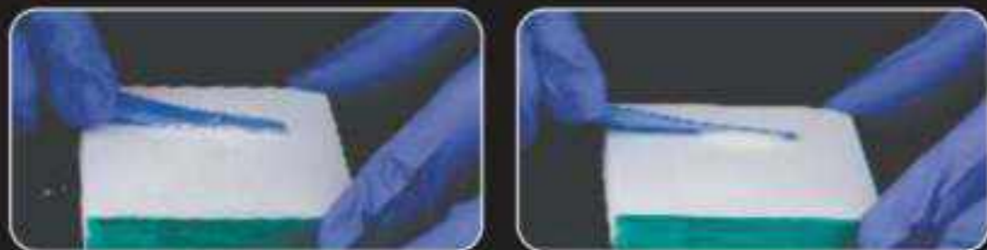
Fig. 10.21, 10.22: The second increment of powder is then spatulated until a smooth uniform mix is obtained.
