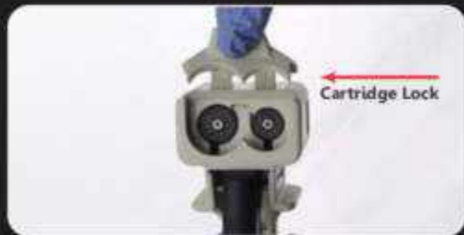
Fig. 5.58: Next, the cartridge lock on the dispenser is lifted up.
