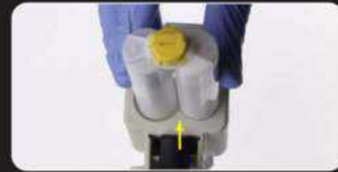
Fig. 5.60: The cartridge is then inserted into this V-notch.
